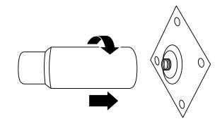
3. Use a Phillips bit to attach the legs with the stainless steel screws supplied. DO NOT OVERTIGHTEN!
