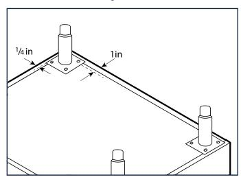
4. Adjust the leveling legs up or down to bring the cabinet to a level plumb position.
