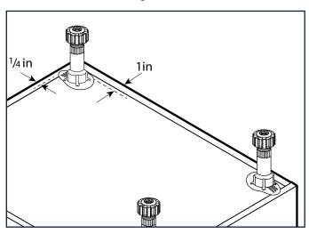
4. Adjust the leveling legs up or down to bring the cabinet to a level plumb position. Use of the longer stems may be needed in this application.
