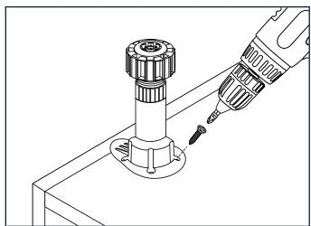
2. Place the 2 back leg brackets 1" from the back edge with the support plate overlapping the end panel – 1/4" from the outer edge.
